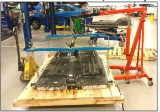
d) Move the replacement EV battery and carefully Move the replacement battery with the Engine place it on the shop floor as a temporary resting point. Remove the Lifting Fixture Kit from the battery.
