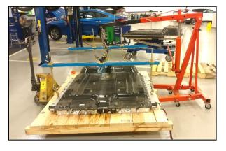
g) Transfer the Lifting Fixture Kit back to install on the replacement battery.
