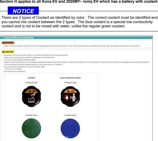
H-1. Fill the P/E cooling system reservoir to the MAX full mark with the following depending on the type of coolant found in the vehicle as identified by color:
