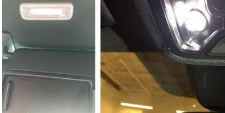
Figure 1. Water intrusion near the headliner.
