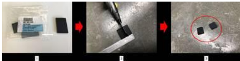
Figure 15. Preparing 2 – 10mm x 10mm pads of 251 201 525 packing.
