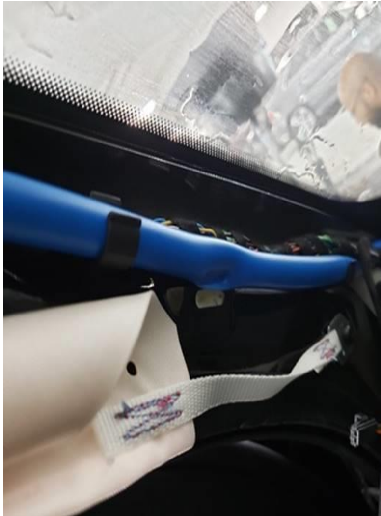
Figure 2. Sunroof drain hose pinched by pillar trim.
