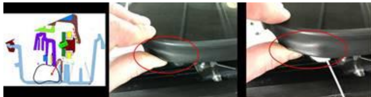
Figure 14. Area of glass panel 'skirt' where bonding agent is to be applied.
