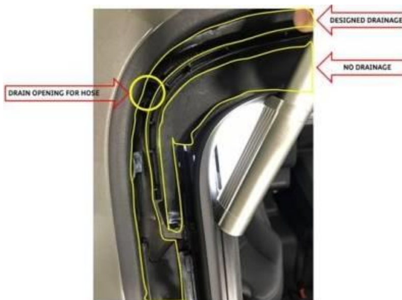
Figure 7. Sunroof water channeling diagram.
