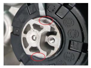
Put lubricating grease with graphite on red marked points as in pictures above.
