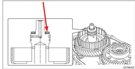
3) Using the Gauge Block, measure the height "A" from the ST end face to the thrust bearing catch surface of the transfer clutch assembly.
