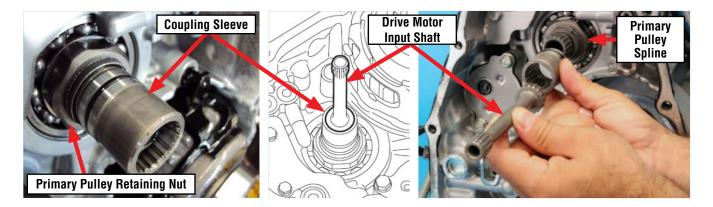
• Once proper spline alignment is confirmed, use some CVT fluid to hold the 6 o-rings in place between the cases during reassembly.
