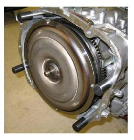
• The torque converter can also be left in place. Either support it from the underside after standing the unit up with a block of wood or use a retainer strap / bracket included with remanufactured and replacement transmission assemblies to keep the torque converter in place.
