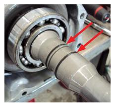
**IMPORTANT:** <u>BEFORE</u> applying any sealer to the cases, always trial fit them together to confirm proper spline alignment between the coupling sleeve, the drive motor input shaft and the primary pulley. The cases are too close together to facilitate turning the primary pulley retaining nut to get the splines aligned properly, especially when there is fresh sealer applied.
