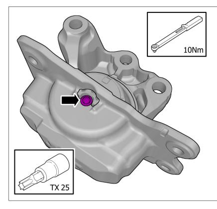
Install the marked component. Tighten the screw.
