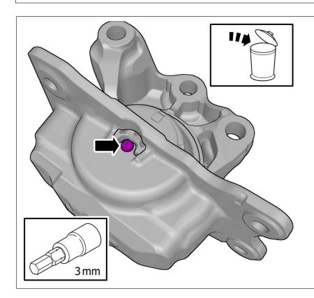
Remove the screw. The part is not to be reused.
