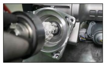
7. Using a torque wrench and SST (B), tighten the shaft nut (C).
