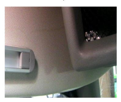
It has been determined that the source of the water is the bolt holes at the center attachment points for the sun visor. A picture of the affected attachment points is shown below.
