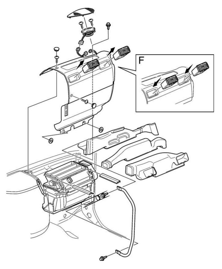
F: The ventilation nozzles must be removed before reinstalling the cover.
