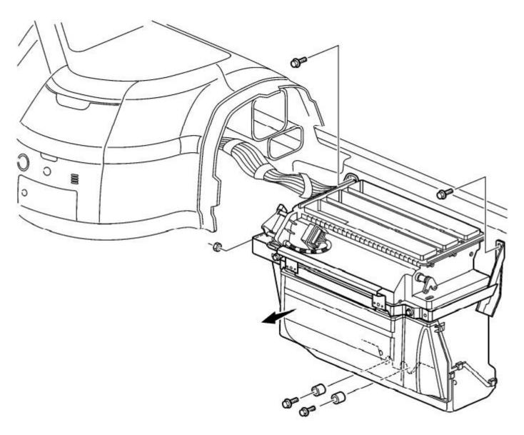
Pull the climate unit backwards and carefully cut off the butyl tape holding the unit in the casing wall.
