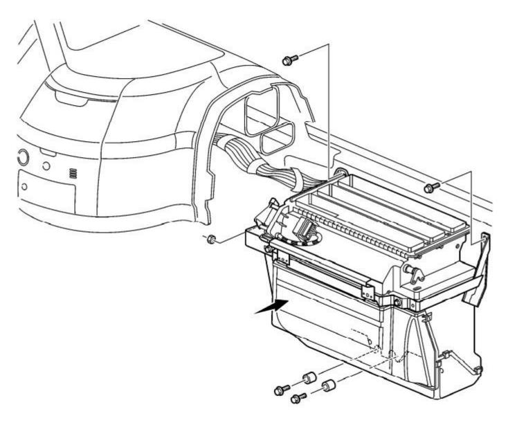
Note: Scrape off and replace the old butyl tape to ensure a good seal.
