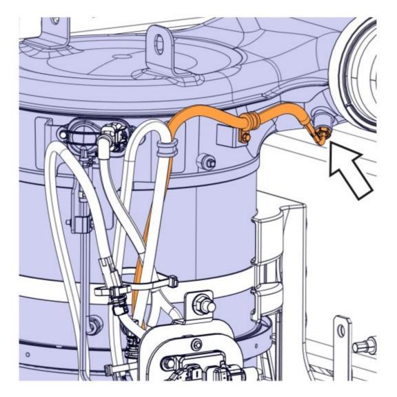
Install the T1 temperature sensor into the port as shown. Tighten the sensor to  $45 \pm 4.5$  Nm ( $33 \pm 3.3$  ft-lb).
