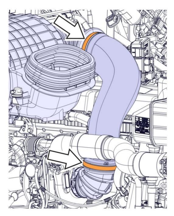
Tighten the intermediate air pipe clamps to  $9 \pm 1$  Nm ( $80 \pm 9$  in-lb).
