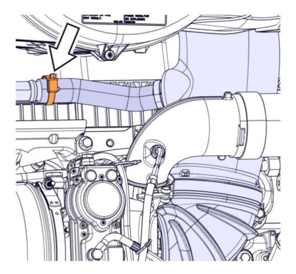
Tighten the air compressor inlet hose clamp to  $3.9 \pm 0.5$  Nm ( $35 \pm 5$  in-lb).
