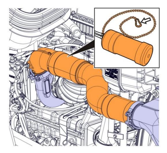
Remove the safety chain from the charge air piping.
