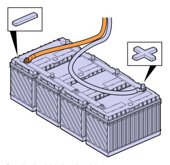
Connect the cable to the battery's negative terminal.
