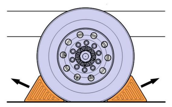
Remove the wheel chocks from the rear wheels.
