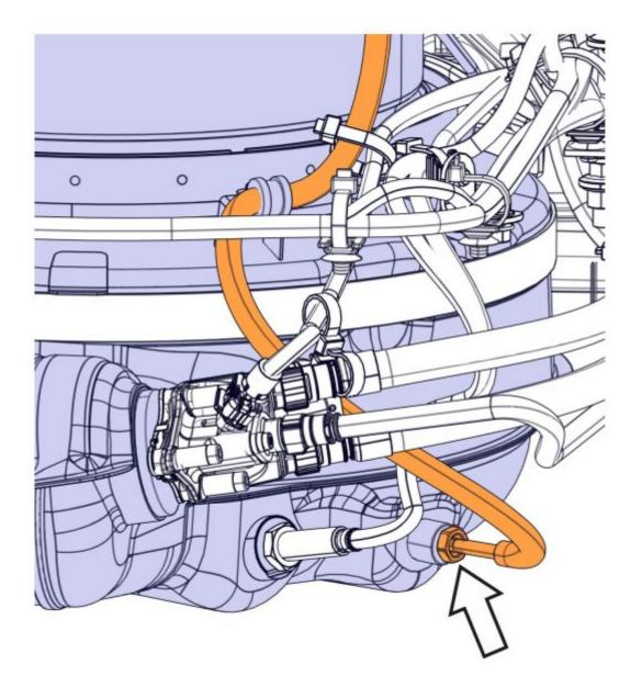
Install the T3 temperature sensor into the port as shown. Tighten the sensor to  $45 \pm 4.5$  Nm ( $33 \pm 3.3$  ft-lb).
