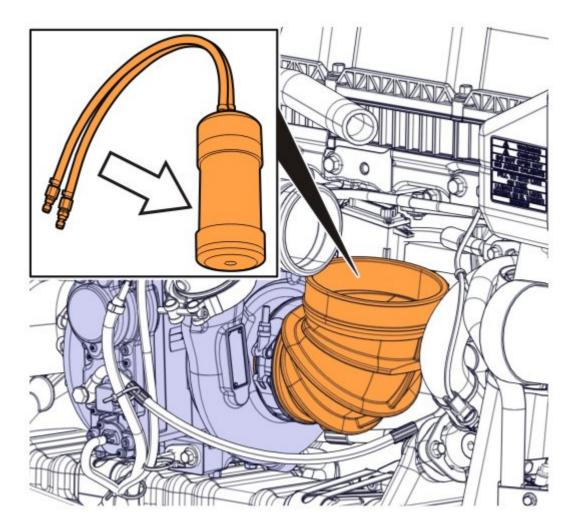
Deflate and remove the air seal from the lower air boot at the engine turbo.
