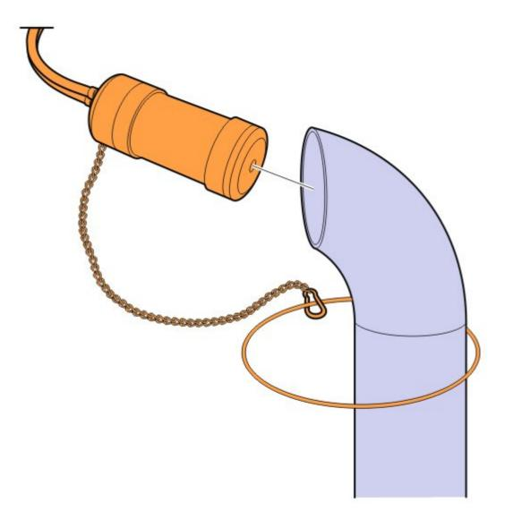
Deflate and remove the air seal from the exhaust pipe.
