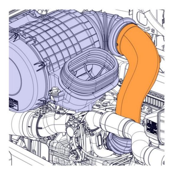
Install the intermediate air intake tube.
