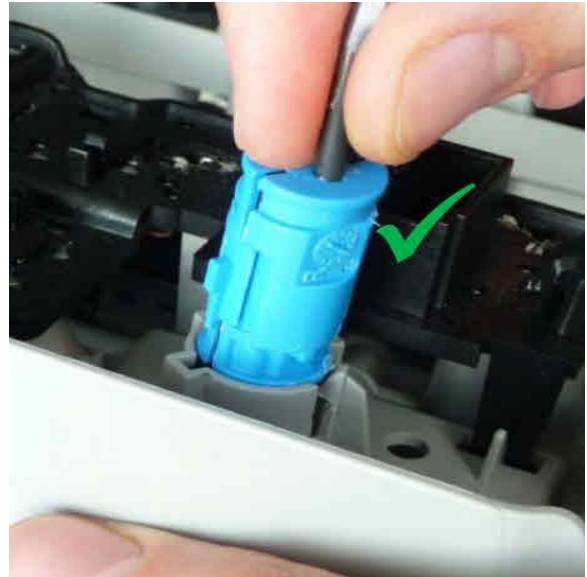
Figure 7. The correct way to install the microphones.
