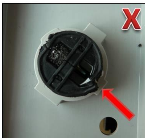
Figure 3. A damaged gasket (microphone needs to be replaced).
