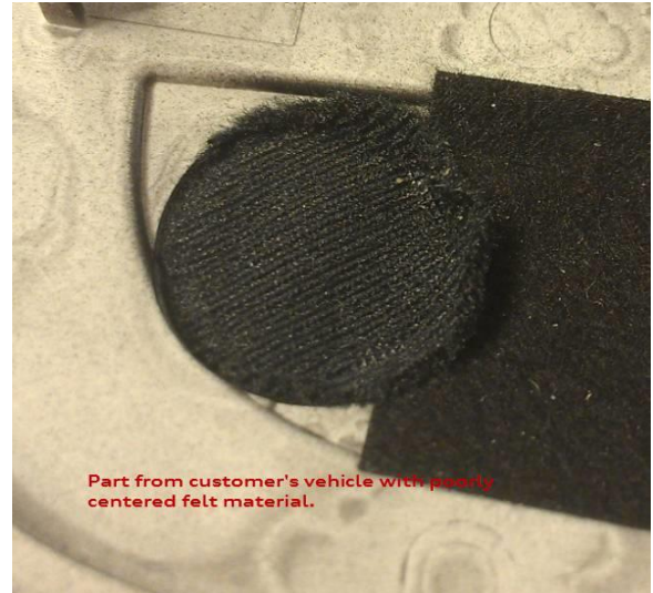
Figure 9. The cloth cover is deformed and uneven.
