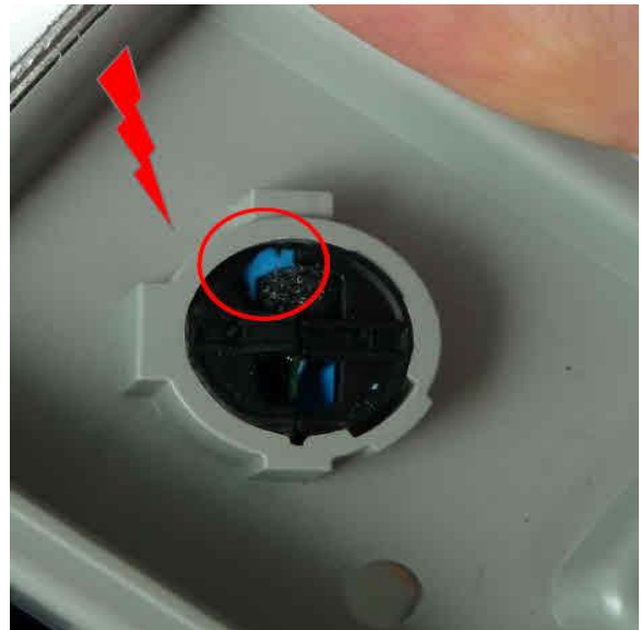
Figure 6. Damage caused by installing a microphone at an angle.
