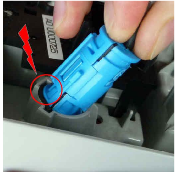
Figure 5. Do not install the microphone on an angle. Always insert the microphone perpendicular to the slot in the dome light module.
