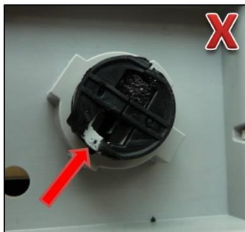
Figure 4. A damaged gasket (microphone needs to be replaced).
