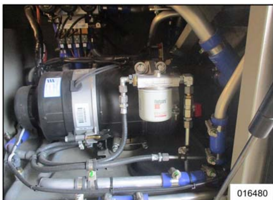
Figure 1: Coolant heater compartment , in front of left drive wheels
