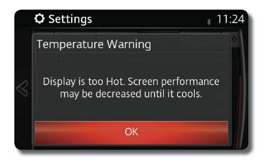
This is a normal screen protection function. **Do not perform repairs for this concern.** Normal screen operation will resume when the screen temperature cools.
