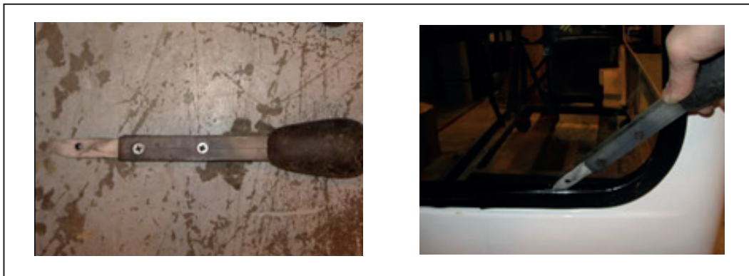
Figure 6 - Flexible Tab Glass Insertion Tool
