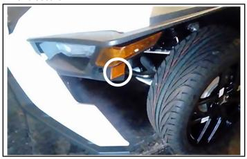
2. Inspect that the passenger's side reflector decal is present and secure.
