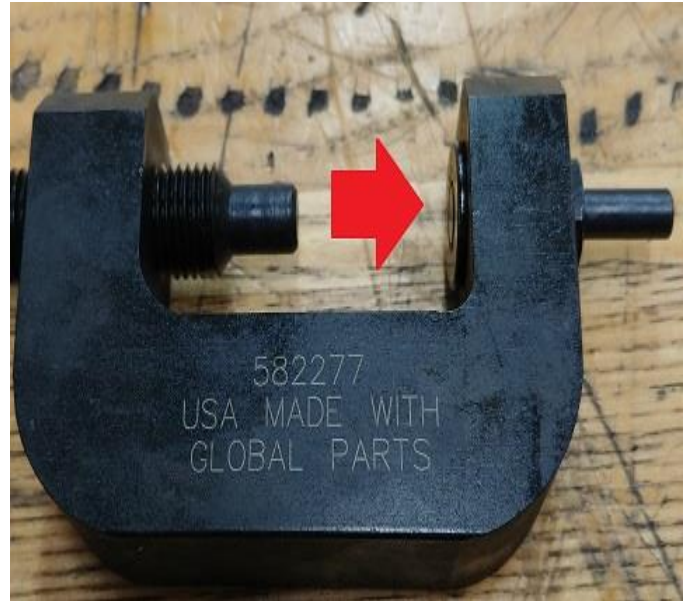
Figure 17. T10172/9 installed in 582277.
