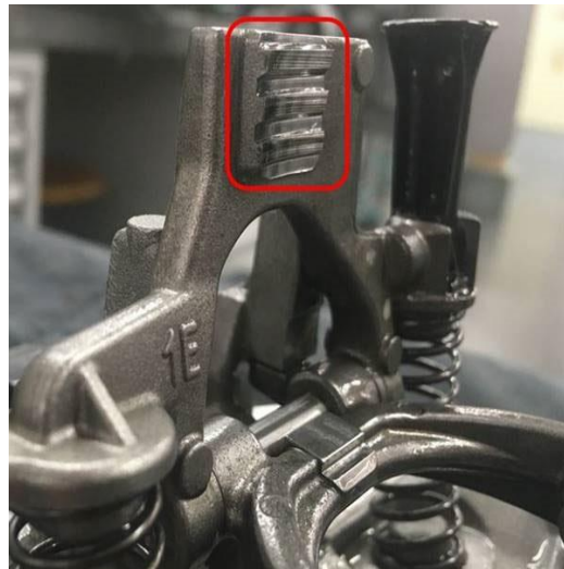
Figure 1. Worn/faulty shift fork.
