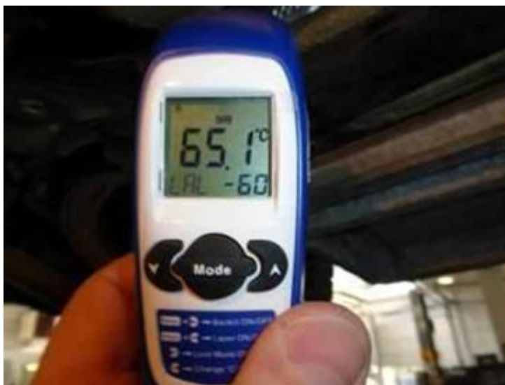
Figure 4. Surface temperature warmed to 65° C (149°F).
