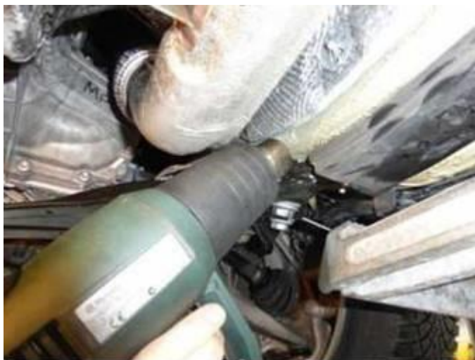
Figure 3. Warming the area of the body near the rear transverse link.
