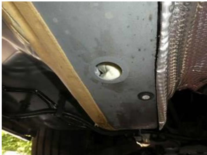
Figure 6. Body plug removed.
