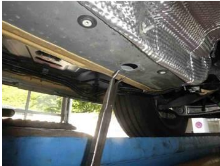
Figure 7. Remove a portion of the acoustic foam.
