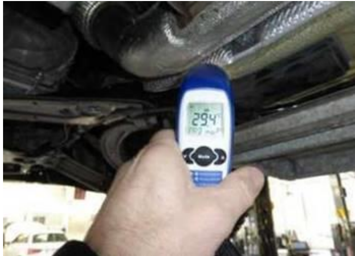
Figure 5. Surface temperature cooled to approximately 30° C (86°F).
