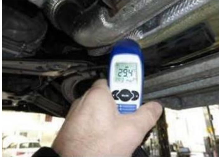
Figure 5. Surface temperature cooled to approximately 30° C.
