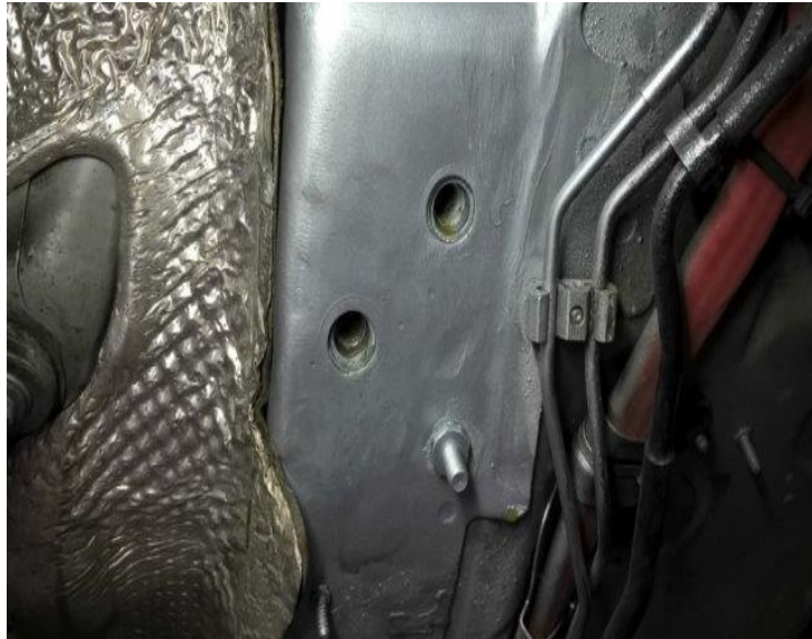
Figure 18. Corrosion protection restored.
