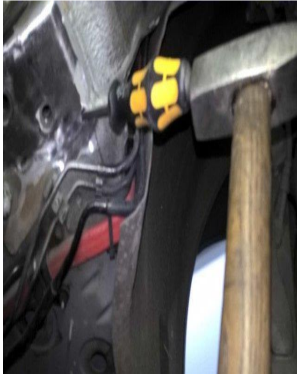
Figure 13. Striking the punch on the nut plate.
