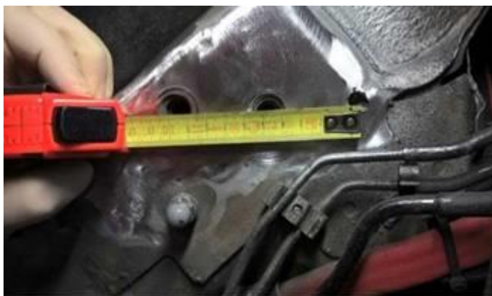
Figure 8. Measuring for the hole's location.
