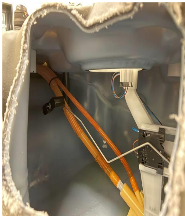
Figure 1. Fuel sender is stuck.
