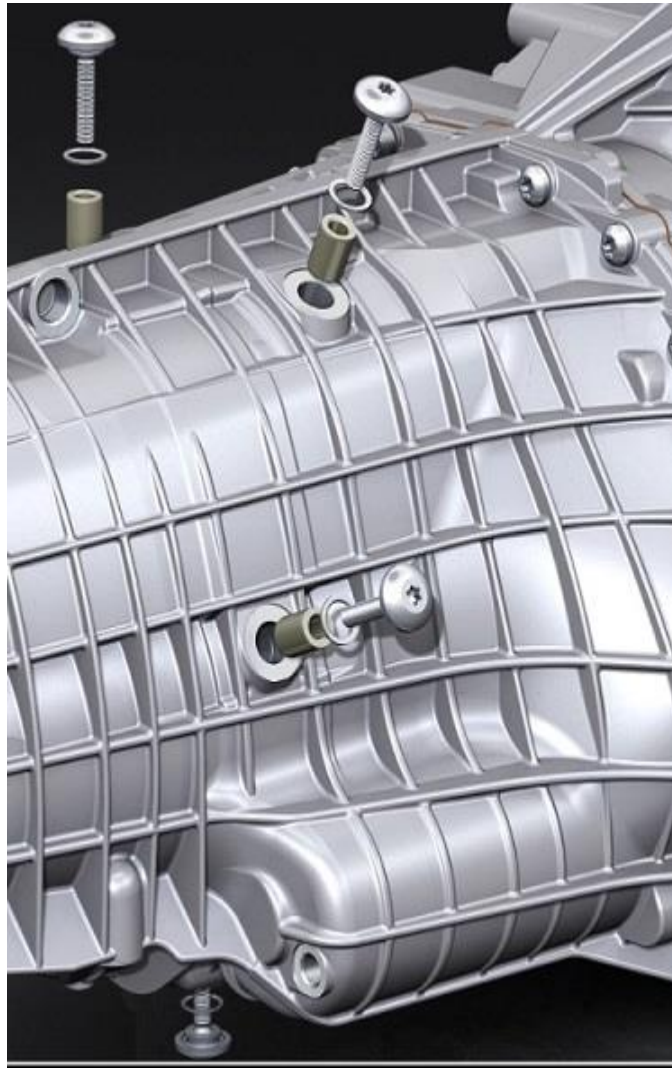
Figure 1. Bearing plate bolts.
