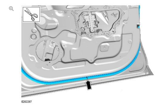
Using a suitable tool, trim the excess length off the newly installed door primary seal so that it meets the other end of the seal on the lower edge of the door.
