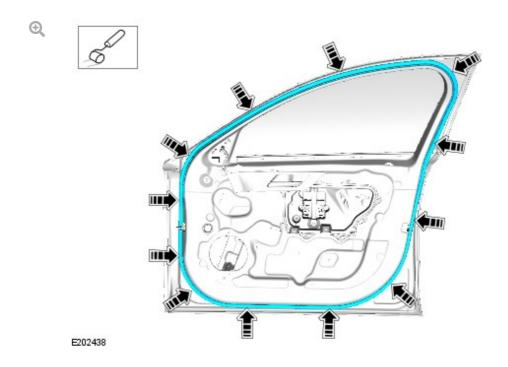
After installing the replacement door primary seal, apply pressure to the seal around the full circumference using a roller or similar to make sure the adhesive bonds to the door.
