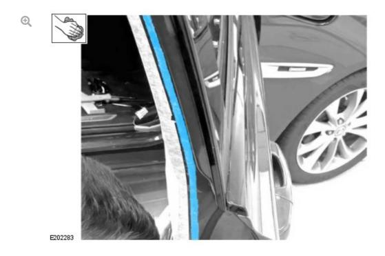
Clean and remove any remaining door seal adhesive from the edge of the door.
