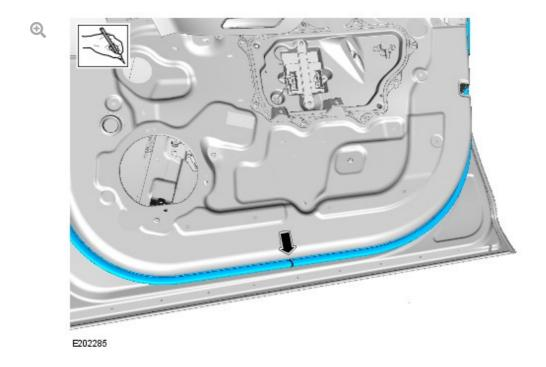
On the lower edge of the door, mark the center position where the two ends of the door primary seal join on the tape already applied.
