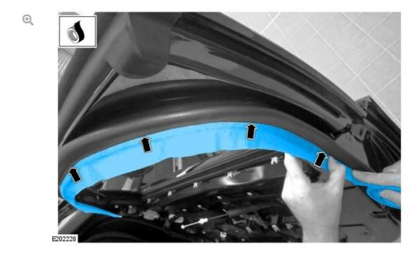
Using a suitable tape, mark the position of the inside edge of the door primary seal following its profile around the whole door.
