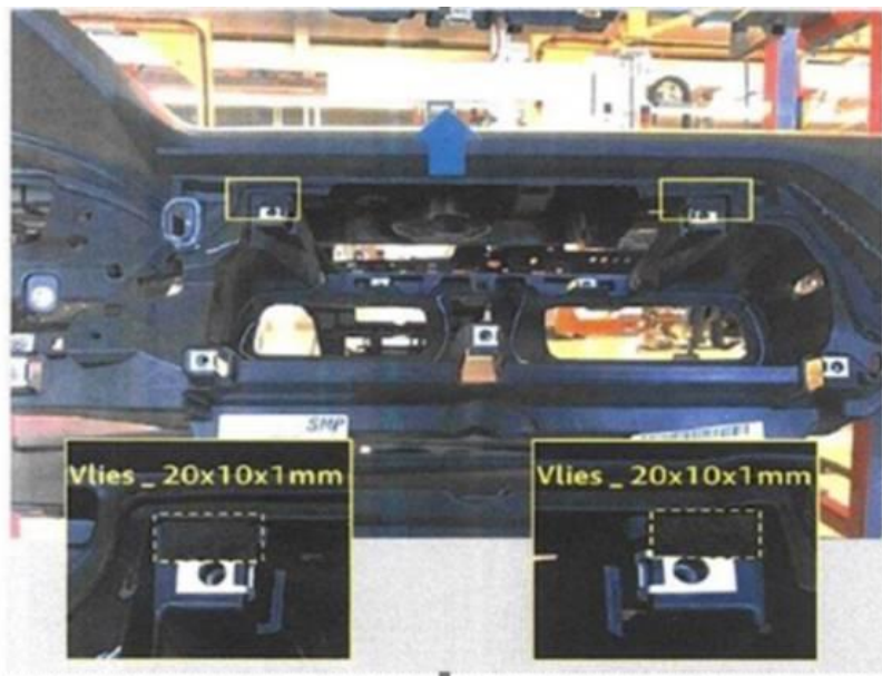
Figure 1. Apply two pieces of felt tape to the dash panel in the area shown.
