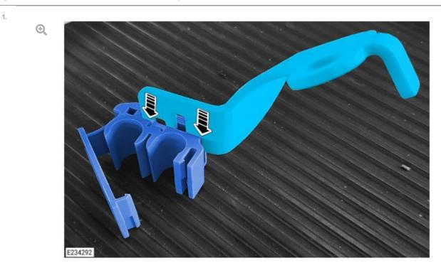
The illustration shows how to install the bracket to the bracket clip as shown.
