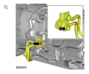
Release the transmission fluid cooler pipes.
