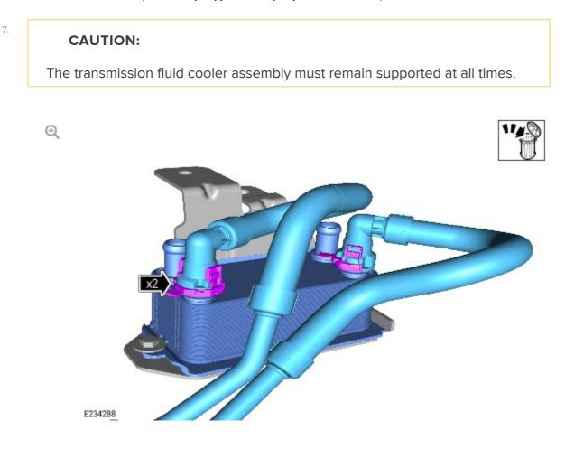
Remove and discard the transmission fluid cooler pipes.
