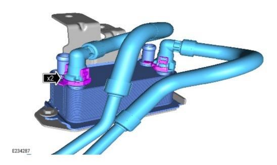
Install the new transmission fluid cooler pipes to the transmission fluid cooler.
