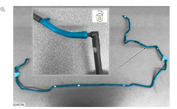
Remove and discard the section of active engine mount vacuum hose.
