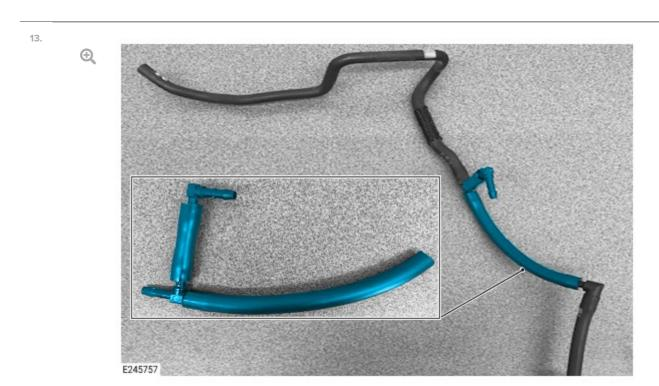
Install the section of active engine mount vacuum hose, as shown in the illustration.
