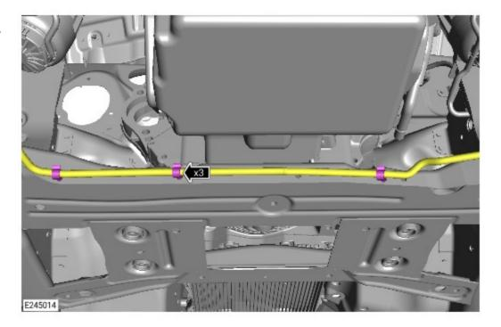
Disconnect the active engine mount vacuum hose from the fasteners.
