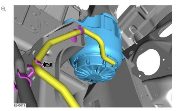
Disconnect the active engine mount vacuum hose from the fasteners.
