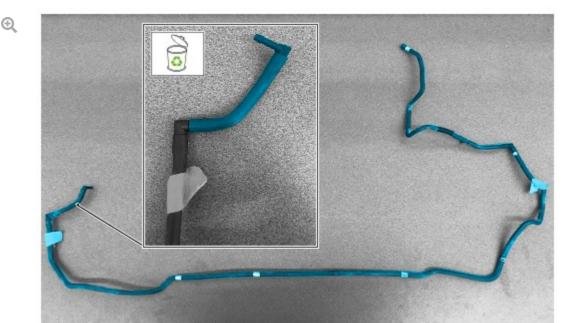
Remove and discard the section of active engine mount vacuum hose.
