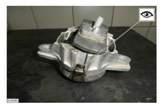
Example of an excessively worn and/or leaking active engine mount.
