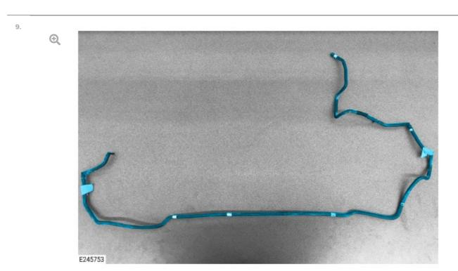
The illustration shows the active engine mount vacuum hose removed from the vehicle.
