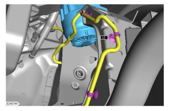
Disconnect the active engine mount vacuum hose from the fasteners.
