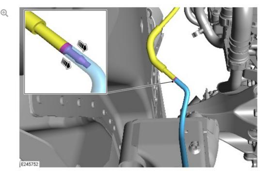
Separate the active engine mount vacuum hose at the connector shown in the illustration.
