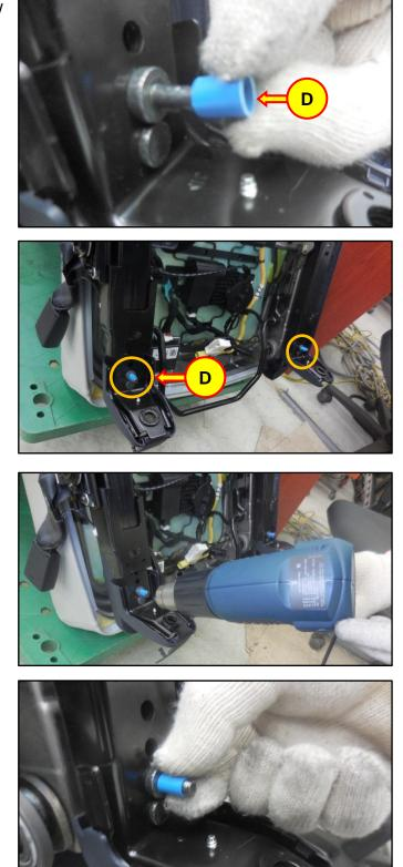
7. Use a heat shrink gun to heat the location pin tubes.
