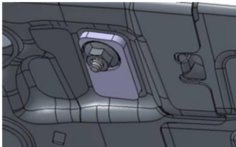
Figure 7. Left side reinforcement plate installation on the Q5.
