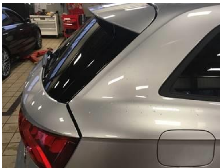
Figure 1. An out of alignment rear lid.
