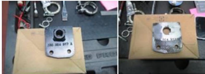
Figure 9. WHT 007 853 reinforcement plates modified.
