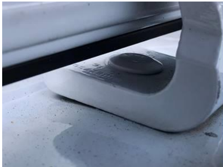
Figure 4. Rear lid hinge mount distorted.
