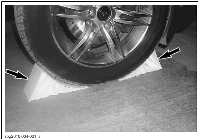
WHEEL CHOCK INSTALLATION, EACH FRONT WHEEL
