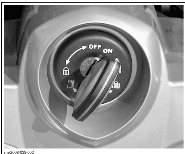
TYPICAL - IGNITION KEY ON
