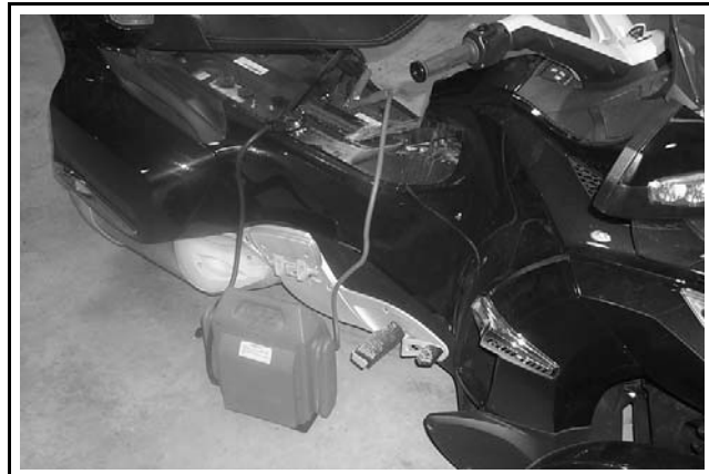
CONNECTION AT BATTERY POSTS UNDER SEAT
