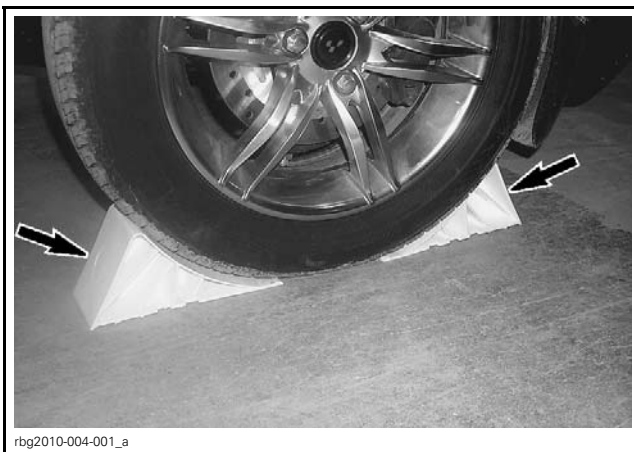
WHEEL CHOCK INSTALLATION, EACH FRONT WHEEL
