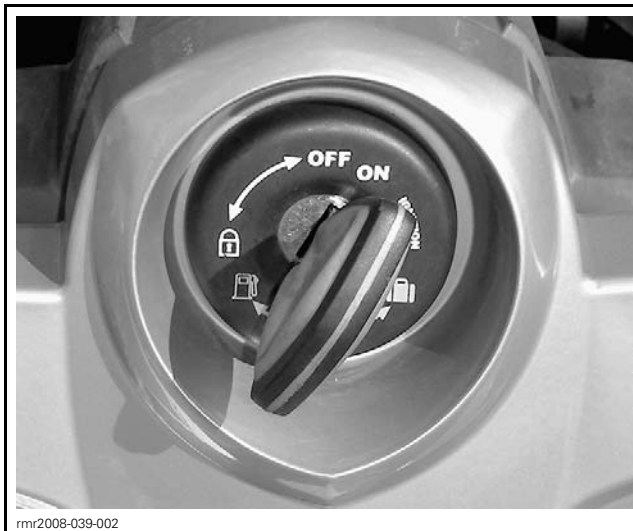
TYPICAL - IGNITION KEY ON
