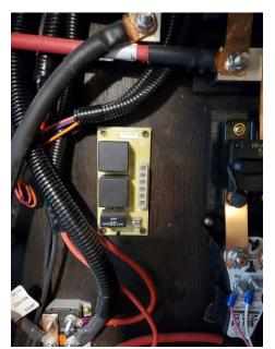
2. Install relay block just above the breakers. As shown in the pictures to the left
