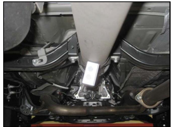
Figure 12. INCORRECT Placement of Digital Angle Gauge
