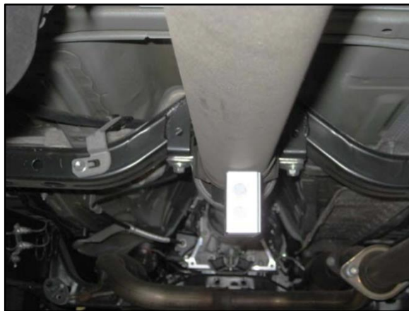
Figure 11. CORRECT Placement of Digital Angle Gauge
