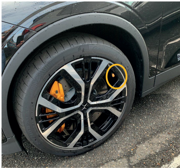
Figure 7. Performance wheel with Brembo brakes and gold valve stem cap. Valve stem caps should be added at PDS if not installed already
