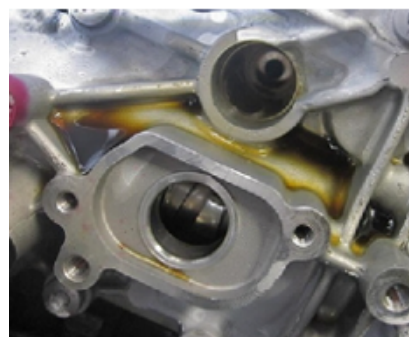
Fault type 2: Cylinder head cover leaking
