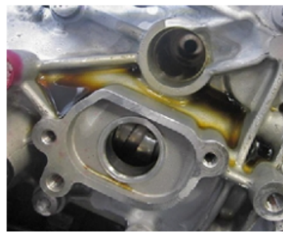
Fault type 2: Cylinder head cover leaking
