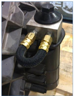
FIGURE 4: VOLVO 9700 - OIL CIRCULATION LOOP
