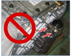
Figure 5: DO NOT BLOCK THE CONNECTION PORTS AT THE TOP OF THE OIL FILTER HOUSING
