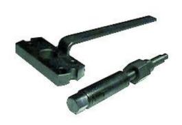
Use: For removing rear axle drive
