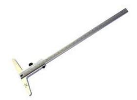
Use: For checking the height of the torque converter
