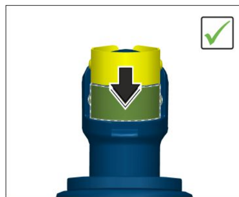
Installing safety clips
