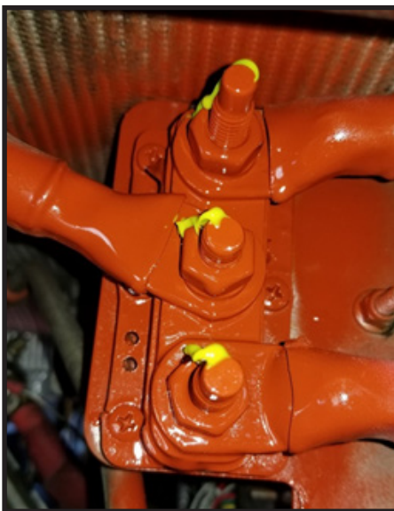
Figure 12 - Dolph ER-44 and Yellow Torque Seal Applied
