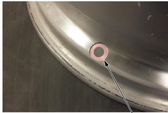
VALVE BORE INSIDE SURFACE
