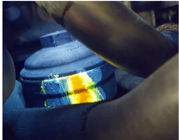
Figure 1. Example of finding a leak using the additive and UV lamp.
