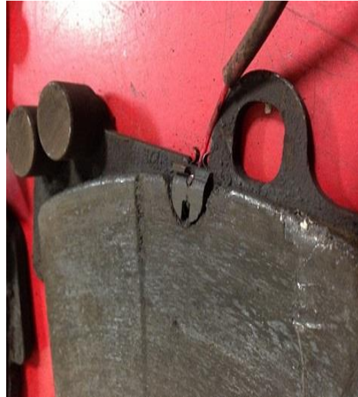
Figure 7. Worn brake pad.
