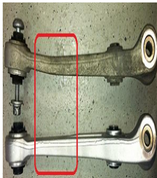
Figure 9. Damaged suspension link.
