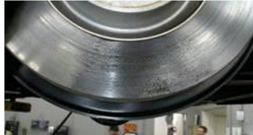
Figure 5. Pad marks on the brake disc.
