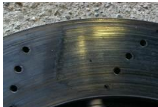
Figure 2. Deposits on the brake disc.
