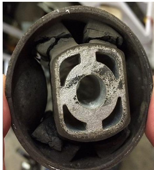
Figure 8. Damaged suspension bushing.
