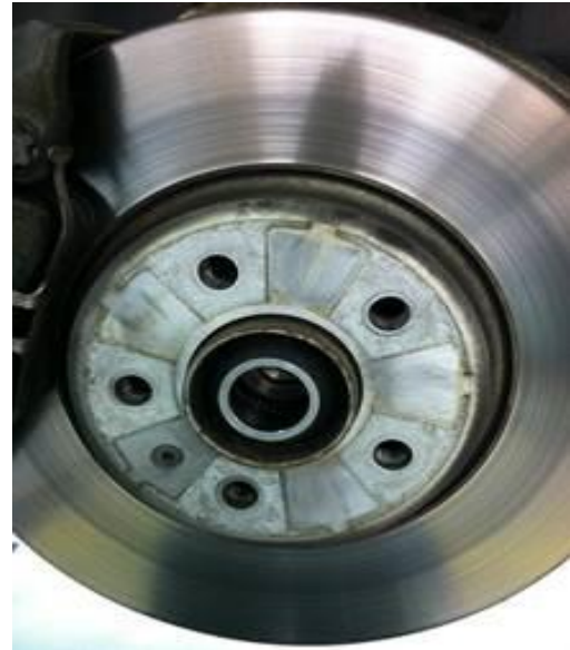
Figure 3. Brake disc with heat marks.
