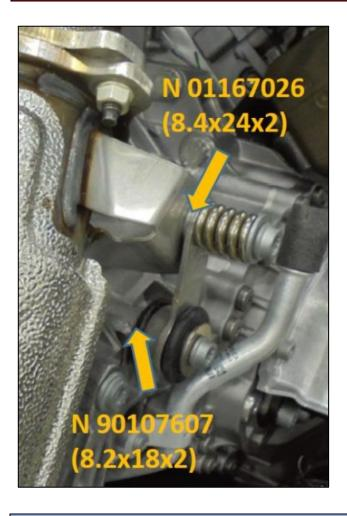
• Install spacer washers to the exhaust bracket.
