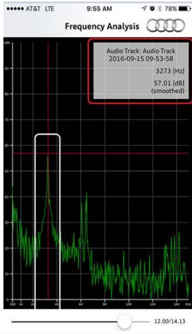
Figure 10. Typical brake squeal frequency recording.
