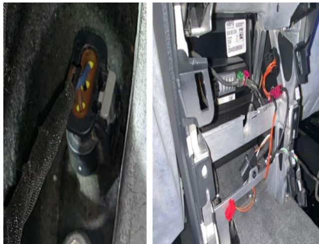
Figure 2. G28 crank sensor harness tight (left), Q5 Wireless charging pad harness tight (right).
