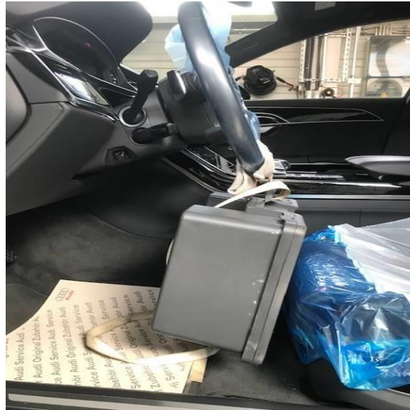
Figure 2. Weight necessary for steering adjustment.
