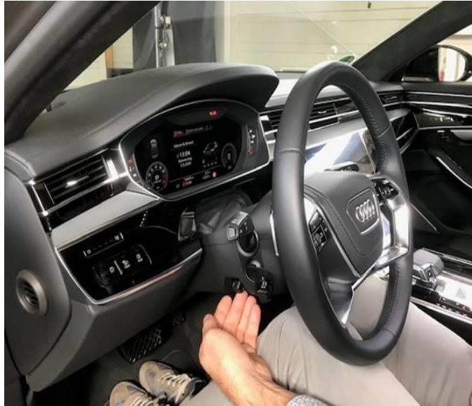
Figure 1. 40 kg force pushing steering wheel upward.
