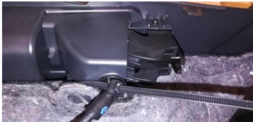
Figure 2. The Bowden cable reinstalled and secured with tie wrap.
