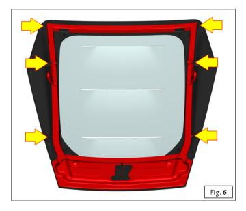
Remove the 4 screws fastening the window to the frame. Keep the original screws and the relative seals as they will be reused to fasten the new Lexan window - Fig.7.
