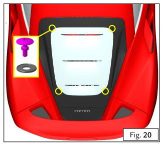
> Wait at least 4 hours and then use heptane to clean off any residue of sealant from around the engine compartment lid screen.
