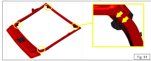
> Fit the frame of engine compartment lid in its seat - Fig.12.
