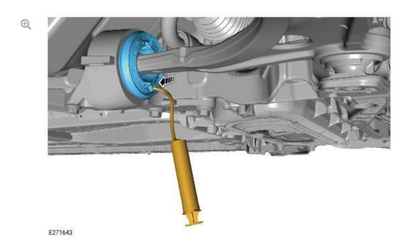
Insert the syringe and length of tube into the fill port.
