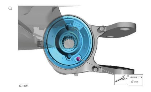
Drill a hole through the rear hydrabush fill port using a 6 mm diameter drill bit, to a depth of no more than 23 mm.
