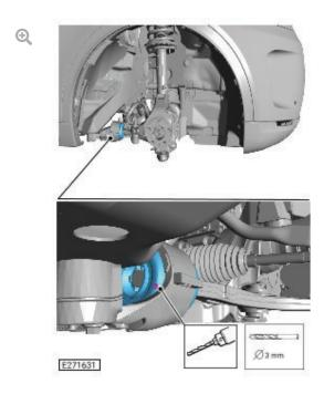
Drill a hole through the back of the hydrabush casing using a 3 mm diameter drill bit, this will assist with the removal of the hydrabush fluid in the next step.
