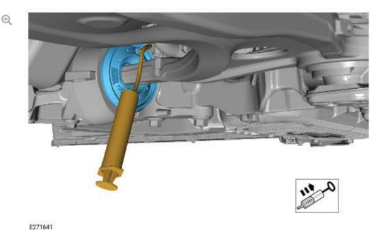
Using the syringe and length of tube, remove as much hydrabush fluid as possible through the hole created in the fill port. A minimum of **50 ml** of hydrabush fluid must be removed before continuing to step 17.
