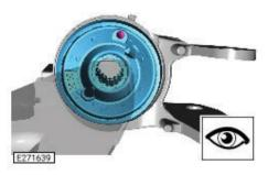
Locate the fill port on the rear hydrabush of the front lower control arm, as shown in the illustration.
