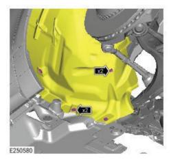
Reposition the front right wheel arch liner.
