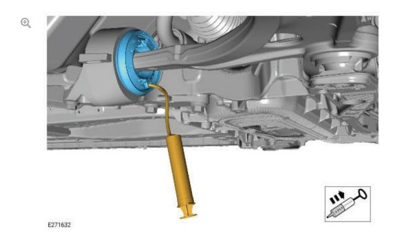
Using the syringe and length of tube, remove any excess degreaser/hydrabush fluid through the hole created in the fill port.
