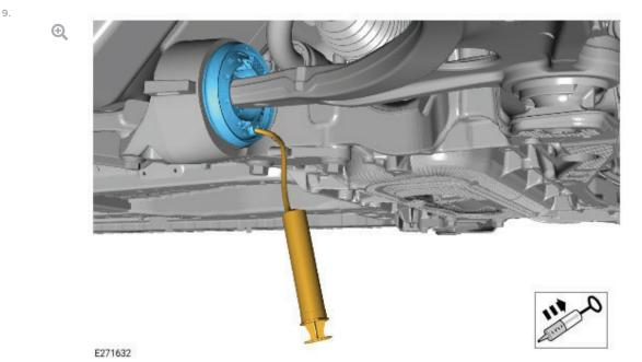
Using the syringe and length of tube, remove as much hydrabush fluid as possible through the hole created in the fill port. A minimum of **50 ml** of hydrabush fluid must be removed before continuing to step 9.
