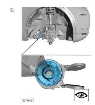
Locate the fill port on the rear hydrabush of the front lower control arm, as shown in the illustration.
