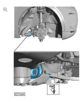
Using a center punch, mark the drill location on the back of the hydrabush casing. This will assist with drilling the hole in the step.
