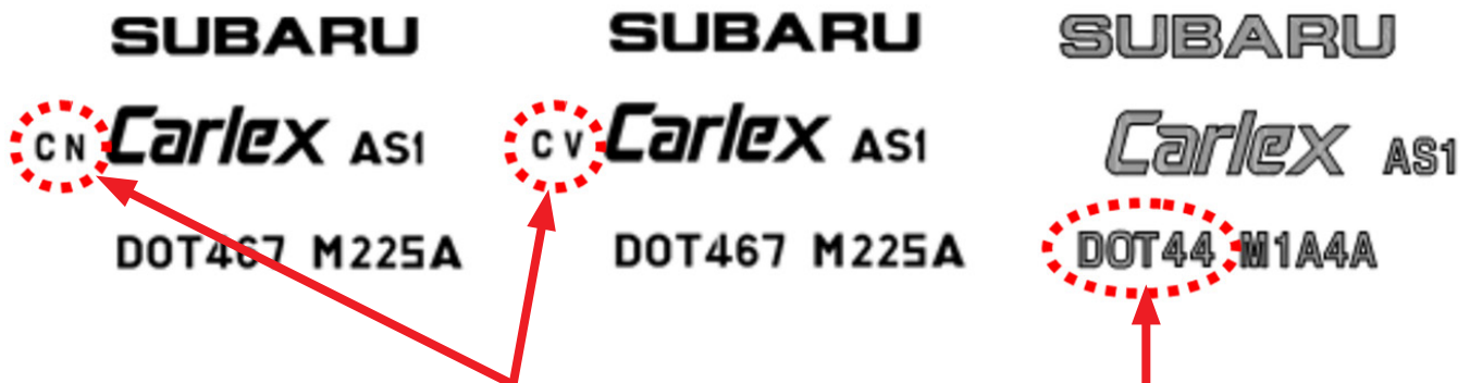
Fig. 2 These 2 production markings can be found on production or replacement part windshields. This marking is found on replacement part windshields only.
