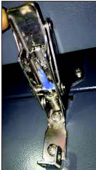
Figure 3 - Apply Thread Locker
