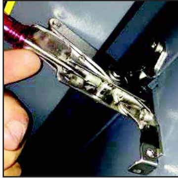
Figure 2 - Loosen the Adjustment Screw
