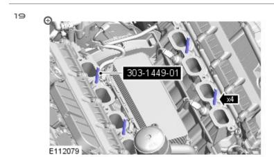
Install the guide pins to aid installation of the supercharger.
