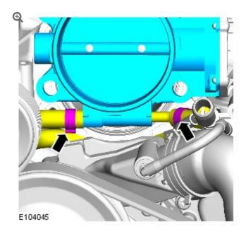
Disconnect the hoses and remove the throttle body.
