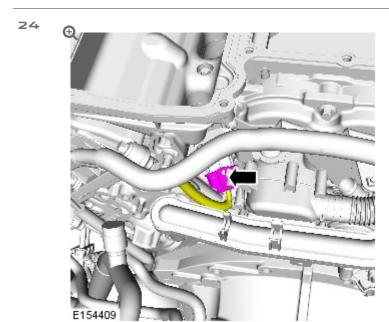
Install the wiring harness.
