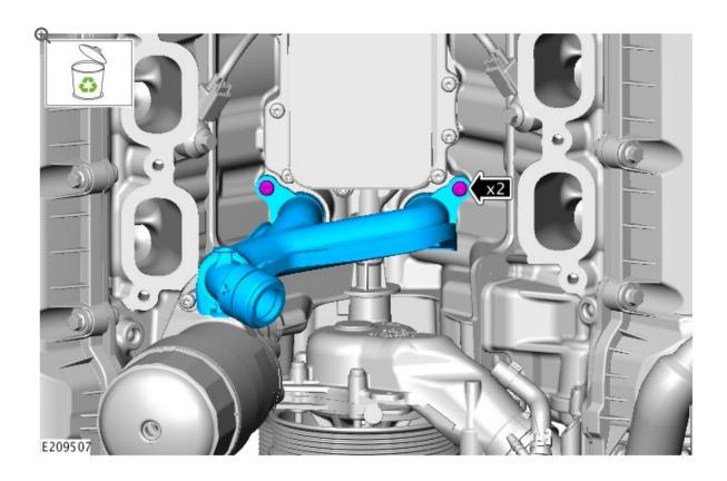
Remove and discard the lower coolant outlet pipe.
