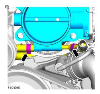
Install the throttle body and connect the pipes.
