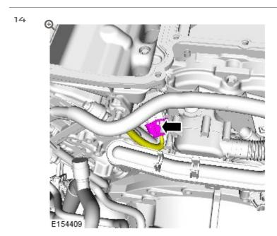
Disconnect and reposition the wiring harness.
