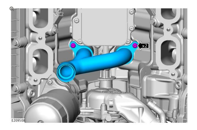
Install the replacement lower coolant outlet pipe.
