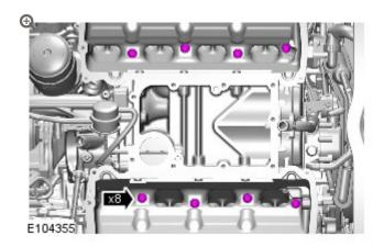
Remove the fasteners.
