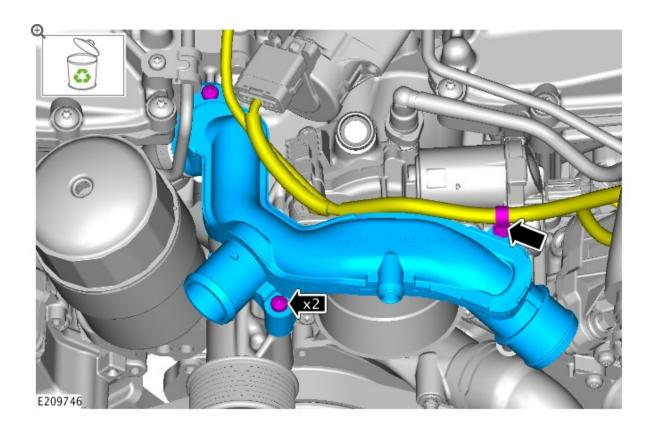
Remove and discard the upper coolant outlet pipe.
