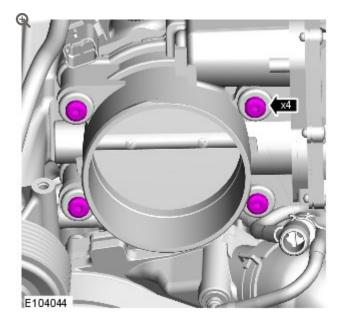
Install the throttle body fasteners.
