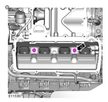
Install the two remaining fasteners into the locations where the guide pins had previously been installed.
