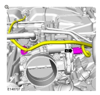
Install the wiring harness to the throttle body.
