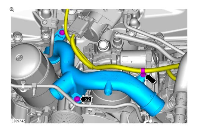
Install the replacement upper coolant outlet pipe.
