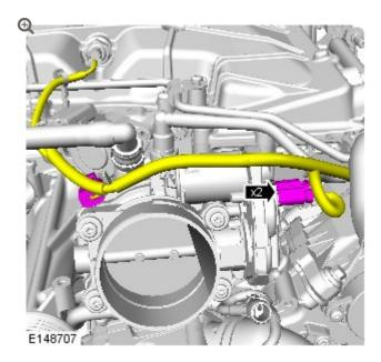
Disconnect the wiring harness from the throttle body.
