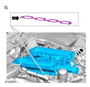
Remove the supercharger assembly.
