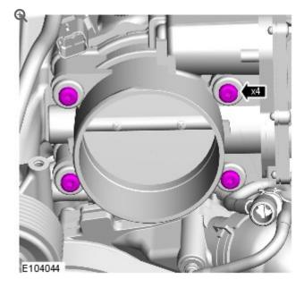
Remove the throttle body fasteners.
