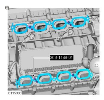
Install new supercharger-to-cylinder head gaskets.
