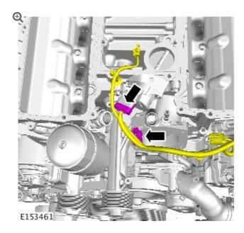
Disconnect and reposition the wiring harness.
