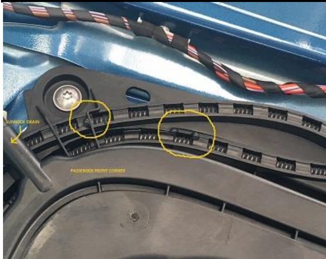
Figure 2: water leaking through sunroof cable guides
