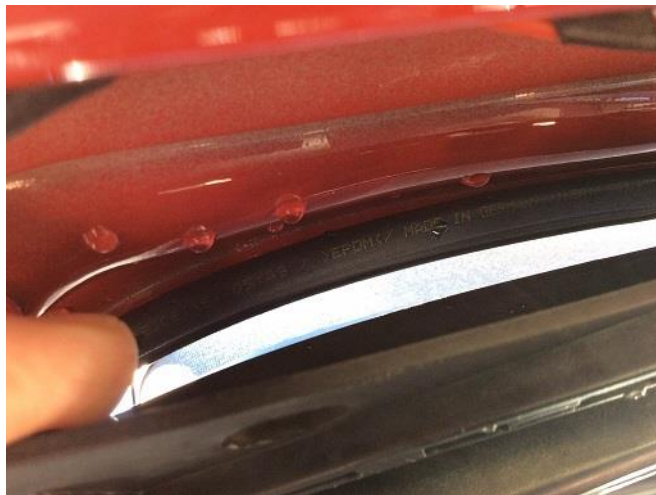
Figure 1: water leaking between sunroof frame and body
